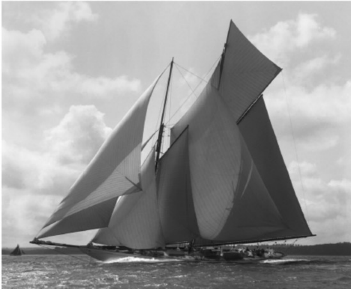
Gaff rigged Schooner, wooden hull, 1900
