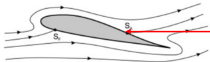
Start of air flow past the wing
