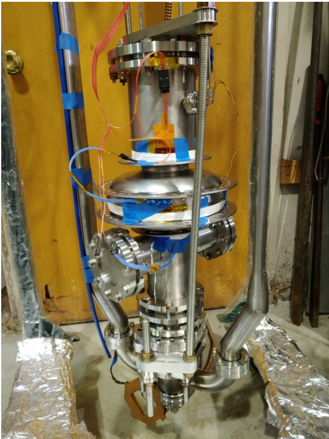
Figure 6.8: LCC1-1 fully assembled onto a test pit insert with sensors and instrumentation added. Cernox sensors are attached at the equator and each iris, while flux gates are mounted vertically at the equator and top iris.
