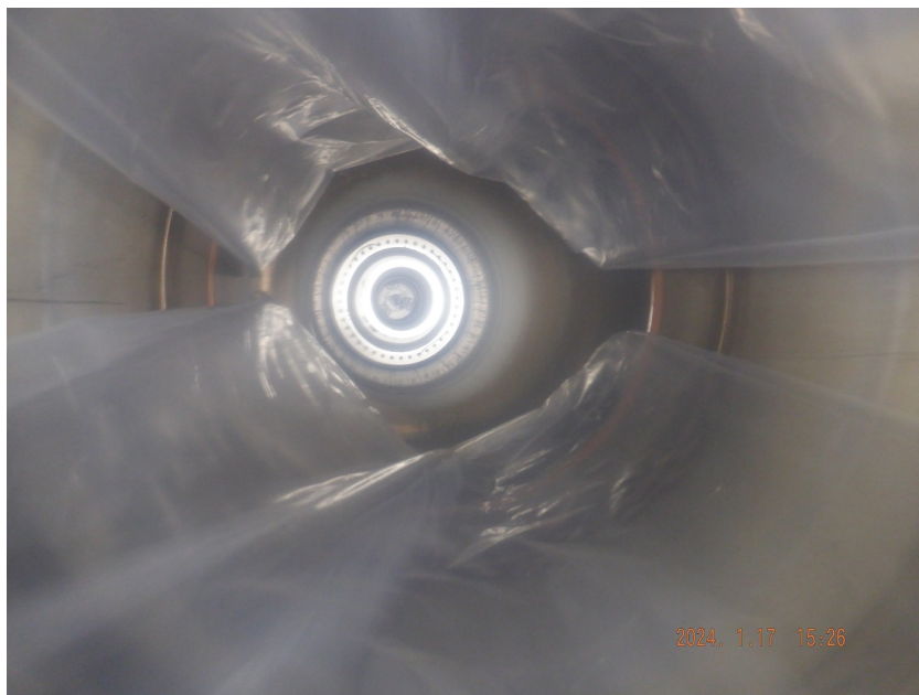
Figure 6.12: LCC1-1 placed in the bottom of the \text{Nb}_3\text{Sn} furnace. Visible at the top and bottom of the image are clean plastic bags used as buffers in the upper stainless steel portion of the furnace. These were added due to the large diameter of the cavity being only slightly smaller than that of the furnace.
